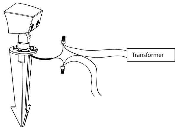
Note: To install multiple fixtures, also connect the power supply wire of each additional fixture to the connection described in 7 of the previous fixture.
