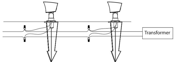
Note: To install multiple fixtures, follow the diagram above
