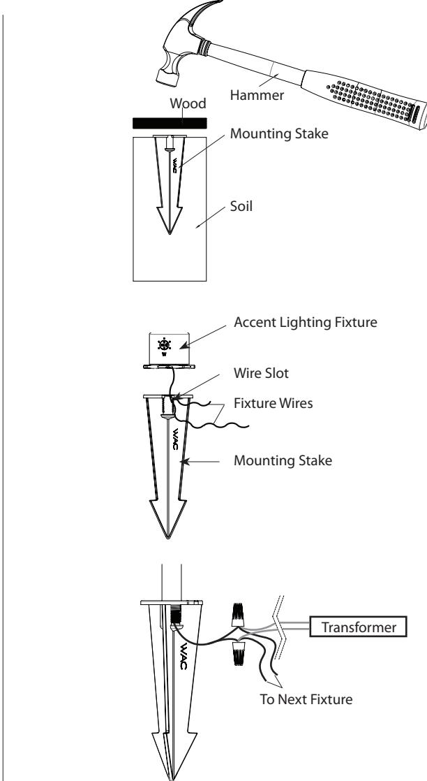
Note: To install multiple fixtures, also connect the power supply wire of each additional fixture to the connection described in 7 of the previous fixture.
