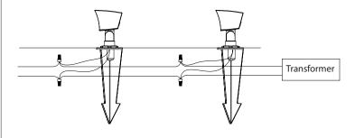
Note: To install multiple fixtures, follow the diagram above
